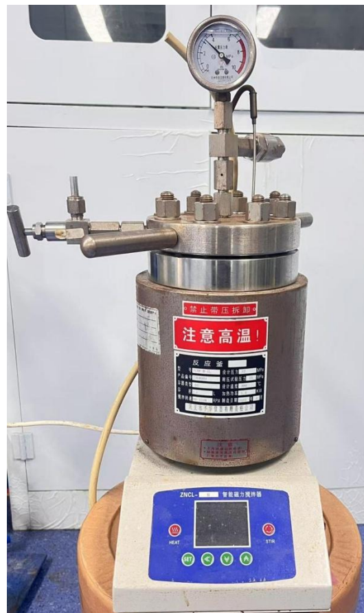
Fig. 2: High-pressure reactor used for TFE addition reactions with temperature and pressure control systems
