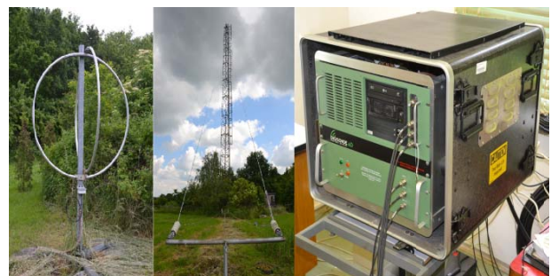
Fig. 5: Digisonde DPS-4D located at the observatory Pruhonice. (Left panel shows receiving antenna, middle panel shows transmitting antenna and right panel shows the computer part of the Digisonde) (Beran et al., 2015)
